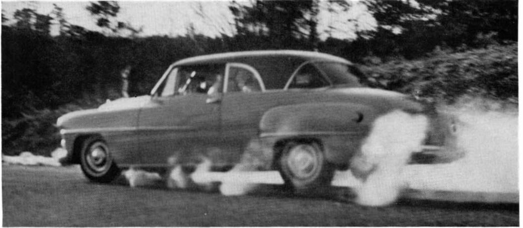
Tires smoke as brakes lock all four wheels at 50 m.p.h. on Dodge Diplomat
